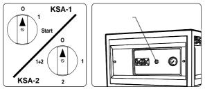
Turn to position 0 Never detach the high pressue hose while the machine is in operation = Position 1, 2 or 1+2.
